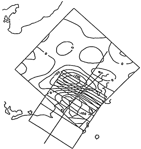
Fig. 1 The magnetic anomaly in the square area and the plan view of a magnetic prism model.
